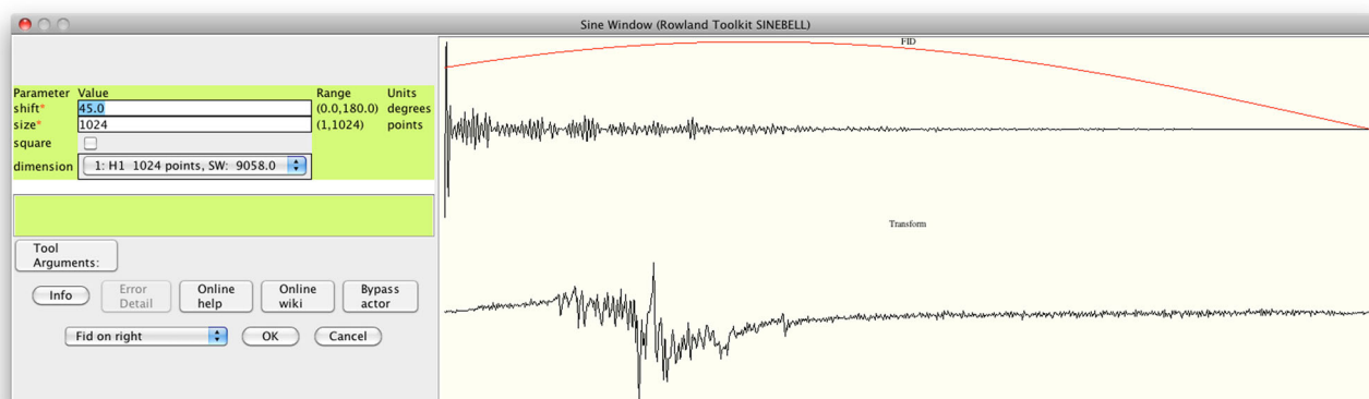
Fig. 6 Interactive parameterization of sinebell apodization shows first data column ( top right, black ), function envelope ( top right, red ), and multiplication ( bottom right )
